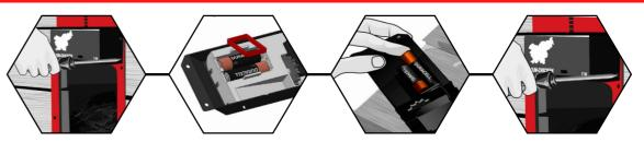
If the door malfunctions or batteries are empty, remove the drive unit by unscrewing the 4 screws using a cross screwdriver (PH2). Take out the battery guard and check/replace the batteries. Check for the + and – signs to insert them correctly. Use only new high-quality batteries. Put back the guard and screw the drive unit back onto the door. Test the door by pressing the button.
